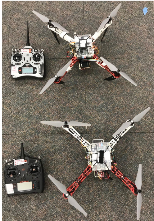
Figure 4-4: Quads with controllers (new quad is bottom quad, it has thinner top plate and black ESCs)
